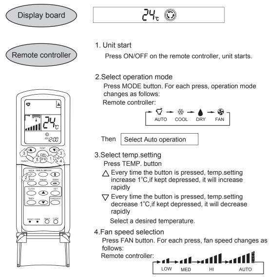
Air conditioner is running under displayed fan speed. When FAN is set to AUTO, the air conditioner automatically adjusts the fan speed according to room temperature.
